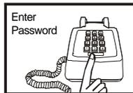
4. After entering the correct password, you can follow the "Phone Command" instructions to perform the required tasks, such as disarm, turn on / off devices or check the system status etc. For further information of how to control the system remotely, please refer to the next section, "Remote Operation by Telephone".
