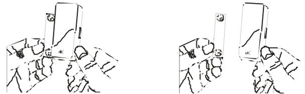
When the magnetic contact is closed, the receiver will not beep.
