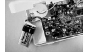
The battery life, (9 volt alkaline battery), is approximately two years if used only for backup.
