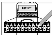
Each switch of this transmitter has 3 positions (" + ", " 0 ", " - "). If the switches of your existing transmitter (Stanley®,
