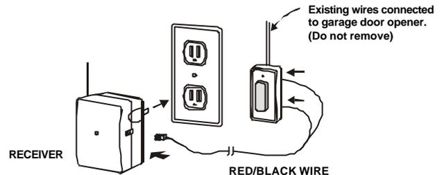
*Note: Alternative wiring options are available, the receiver can be connected directly to the opener's motor. Please contact customer service for further information regarding alternative wiring options.*
