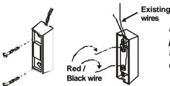
*Note: There should be another pair of wires connected to the 2 terminals already. Do not remove/disconnect these existing wires.*
