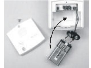
Insert 9V alkaline battery to the sensor
