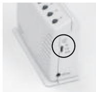
The buzzer can be disabled by switching to the "OFF" position.
