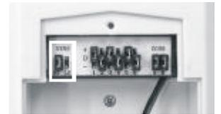
Sensitivity Connectors on Motion Sensor
