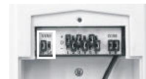
Sensitivity Connectors on Motion Sensor
