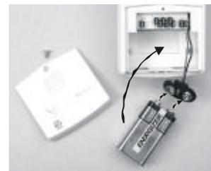
Insert 9V alkaline battery to the sensor
