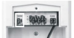
Sensitivity Connectors on Motion Sensor
