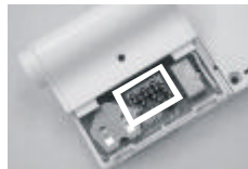
Code connectors on sensor
