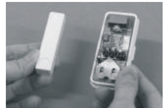
When the magnetic contact is broken (open), the receiver will beep and a LED will flash.
