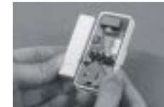
When the magnetic contact is closed, the receiver will not beep.
