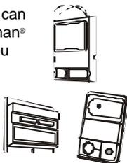
If your Chamberlain®, LiftMaster® and Sears Craftsman® Multi-Function Wall Console has more than 2 wires, the Skylink® GT-100R should be installed in parallel with the original Multi-Function Wall Console. Connect the 2 wires from the GT-100R to the 2 terminals marked “RED” and “WHT” on your existing Multi-Function Wall Console. Polarity DOES NOT matter. *Note: Do not remove the existing wires from your Multi-Function Wall Console.*
