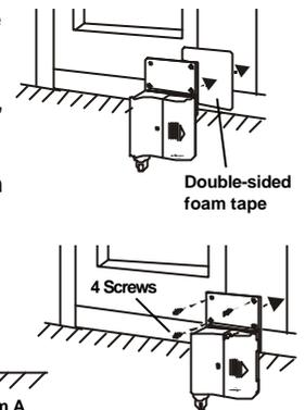
For wooden garage doors, it is recommended to mount the sensor with screws on to the garage door with 3 x 18 screws provided.
