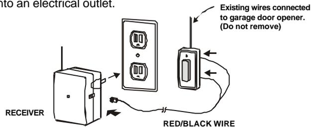
*Note: Alternative wiring options are available, the receiver can be connected directly to the opener's motor. Please contact customer service for further information regarding alternative wiring options.*
