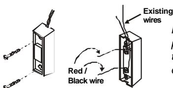
*Note: There should be another pair of wires connected to the 2 terminals already. Do not remove/disconnect these existing wires.*
