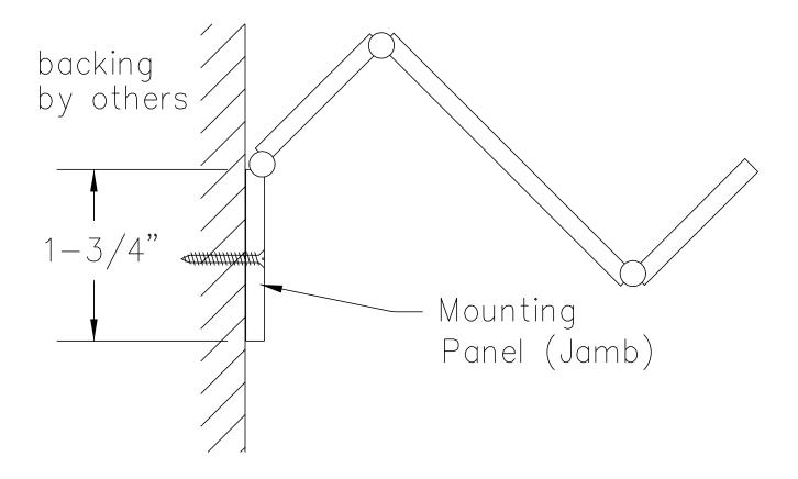
Direction of mounting panel (jamb) varies based on door construction.
